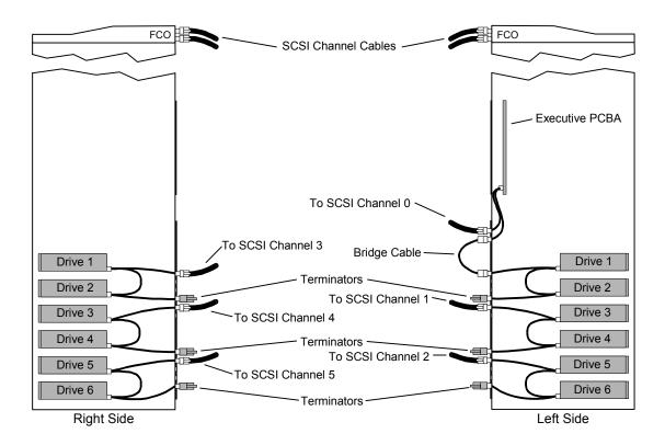
Figure 5-3 TLS-412xxx Cabling Diagram
